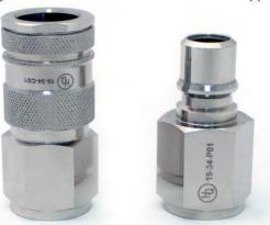
NICKEL PLATED DZR BRASS BODY TOTAL ISOLATION - DOUBLE SHUT OFF O - 35 BAR WORKING PRESSURE
