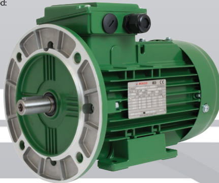
4 Pole, 400V/50Hz, B35 (Foot & Flange) Mounting, IP55 Rated
