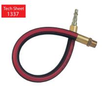
3/8" Bore Rubber-Tech Hose, Plug One End x Male Thread, BSPT
