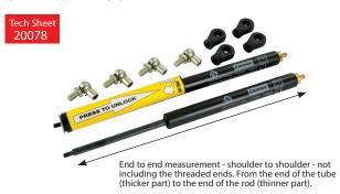
Type: Variable force. Rod Diameter: 8mm Tube Diameter: 18mm Force Range: 100-650N Material: Nitrided steel piston rod, black powder coated steel tube, nylon/steel end connectors.
