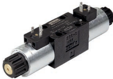
Cetop 3 - 4 Port 3 & 2 Position Solenoid Directional Control Valve - 24-110V
