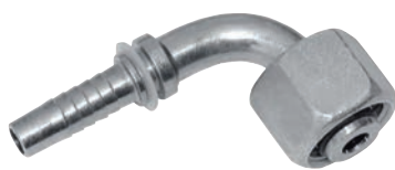
90° Metric Female 24° Cone Seat, S Series, DIN 3865
