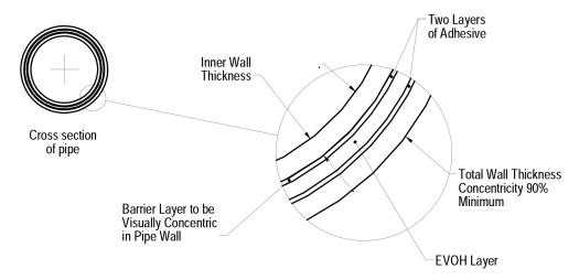
The John Guest Metric five Layer Pex Barrier Pipe is manufactured to BS 7291 Parts 1 and 3 Class 'S' and is Kitemarked for Hot & Cold water and Central Heating.
