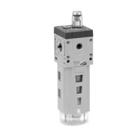
The lubricator allows the nebulization of lubricating oil which is necessary to the functioning of components in specific conditions of use. By means of a regulation screw the amount of oil can be properly adjusted in order to avoid unnecessary overdoses.
